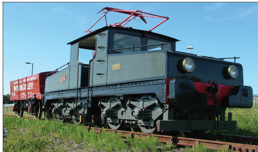
Newcastle's Harton Coal Company pioneered the use of electric traction on its extensive industrial system taking coal and colliery waste to shipping staithes on the River Tyne.
