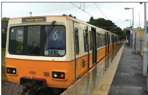
The 48-mile Tyne and Wear Metro, which uses a 1500VAC overhead supply and opened in 1980, has been hailed as Britain's first modern light rail system.
